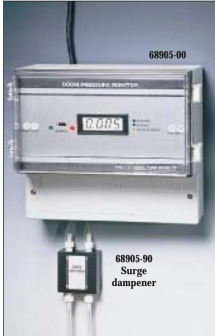
Monitor pressure changes in fume hoods, clean rooms, computer rooms and other isolated areas. Diaphragm actuated capacitance sensors detect pressure changes in the low differential ranges. If air pressure decreases in the monitored area, this transmitter will display negative room pressure and trigger the built-in alarm relay.
